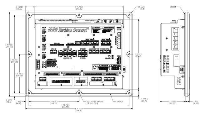
Figure 4. 505 Dimensions (Do not use for construction)
