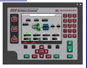
The control's special PID-to-PID logic allows stable control during normal turbine operation and bumpless control mode transfers during plant upsets, minimizing process over- or undershoot conditions. The 505 controller senses turbine speed via passive or active speed probes and controls the steam turbine through one or two (split-range) actuators connected to the turbine inlet steam valves.
